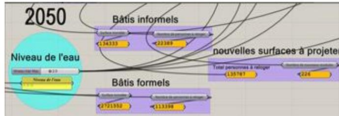
Figure 3: Parametric model evaluating the flooded surfaces in the district of El-Harrach in Algiers, the number of people to be rehoused and the new surfaces to be built according to the rise of water.
